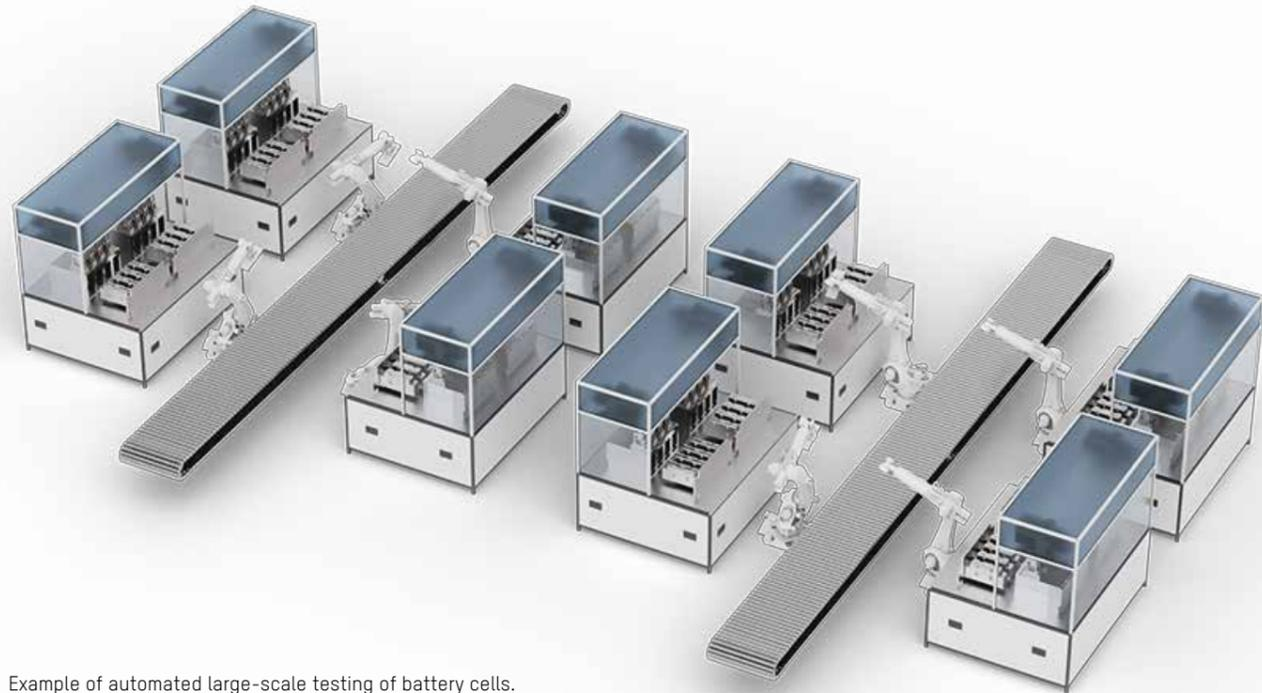
Example of automated large-scale testing of battery cells.
